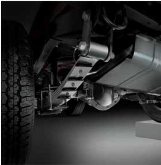
*Above: The mechanical locking differential provides enhanced traction on loose and slippery surfaces without the need for pushbuttons, shift throws or other interventions.*
